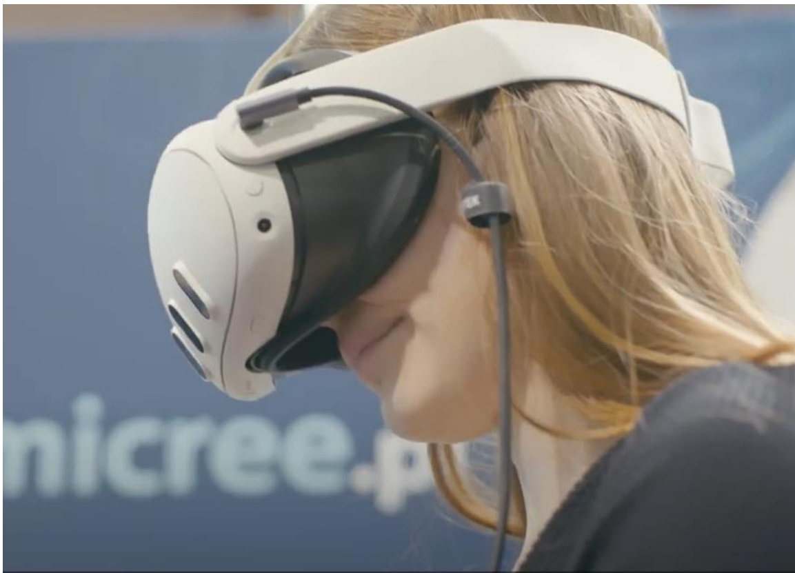
Figure 1. HMD (Oculus MetaQuest 3) connected via USB to external power source as a precaution from the battery running low.
